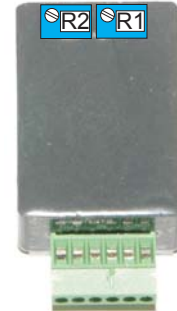
LOCATION OF CALIBRATION TRIM POTS, TOP VIEW
