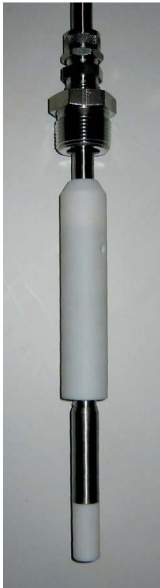
SHIELD PUSHED UP FOR CLEANING
