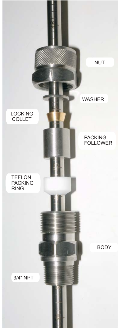
EXPLODED VIEW, 3/4" 300 LB SLIDING FITTING
