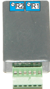
LOCATION OF CALIBRATION TRIM POTS, TOP VIEW
